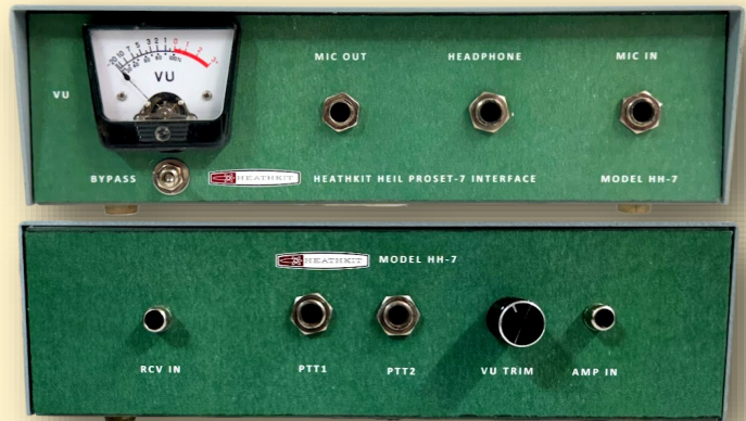
Box repurposed as a mic impedance match box
