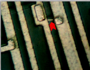
Micro-photograph of ESD damage inside a solid state device
