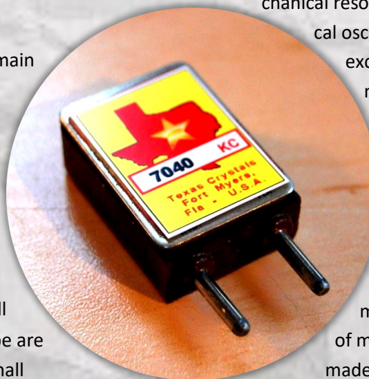
One of many cosmetically restored FT-243 crystals from the collection of Dave W7UUU
