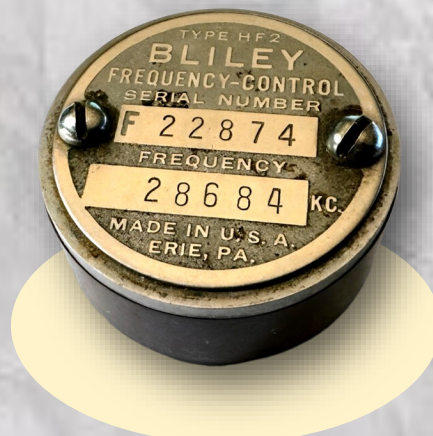
Early Bliley quartz crystal in HF2 mount
