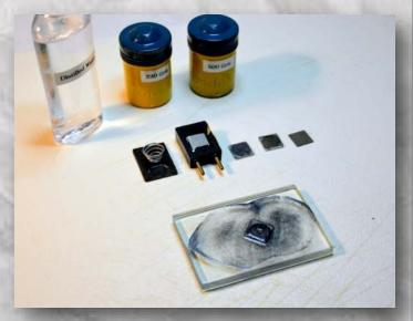
Basic crystal grinding setup: distilled water, 220 & 500 grit, and a thick piece of plate glass. It's not hard—just delicate. Photo by: Dave W7UUU
