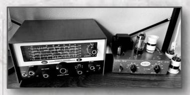
Typical "Novice-era station" - Ameco R5 receiver paired with the iconic Ameco AC-1 single-tube crystal transmitter ca. 1965 From the collection of Dave W7UUU
