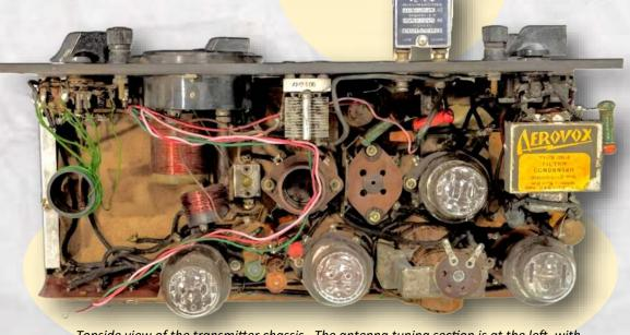
Topside view of the transmitter chassis. The antenna tuning section is at the left, with the green wires being taps off the tank coil. In the center, one tube is missing: the transmitter used push-pull audio for the modulator. Somewhere along the line over the years, one of the type-45 direct-heated triodes got robbed for some other use. The modulation transformer can be seen below the remaining modulator tube. From the W7DK collection—Photo by Dave W7UUU
