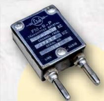
Crystal possibly used was for 1224.375 KHz... in the AM broadcast band (no record exists of what frequency was used)—but this crystal was found in-situ in the transmitter XTAL socket Photos by Dave W7UUU
