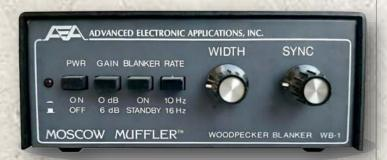
The AEA Moscow Muffler filter was designed to mitigate the effects of the Russian Woodpecker. It was difficult to adjust, in that the width and sync controls had to be set to precisely align with the duration of the pulse, as well as it's spectral width which could vary according to propagation. Additionally, the operator had to figure out if the pulses were 10 Hz or 16, but due to ionospheric effects, could vary. In the end, the Moscow Muffler was a poor solution and was not very effective.
