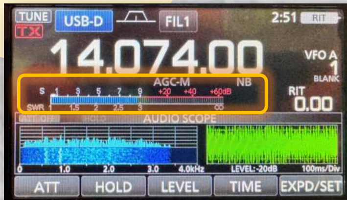
Note the persistent near-S9 noise level across the entire bandwidth of the IC-7300 passband filter even with the Noise Blanker (NB) engaged
