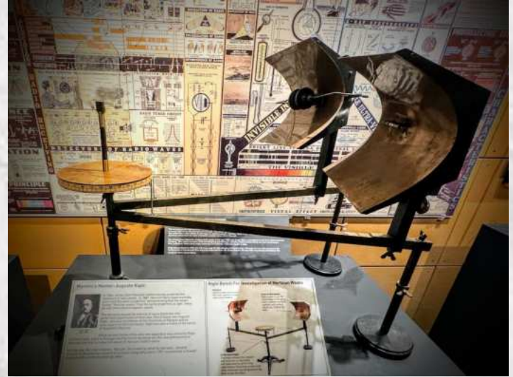
Righi Bench for investigation of Hertzian Waves
