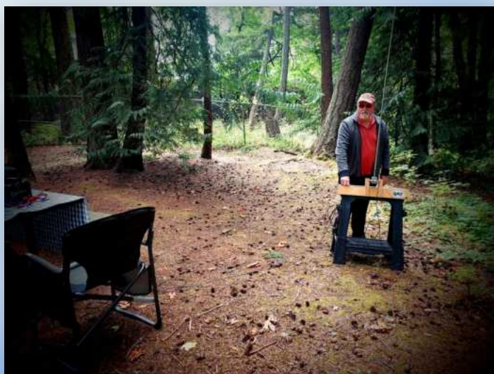
This is me, Dave W7UUU , with my trusty “plastic sawhorse” antenna mount supporting an MFJ-1979 17-foot telescoping antenna that covers 20 meters and up full size and lower bands with the LDG-Z11Pro tuner with my Icom IC-7300
