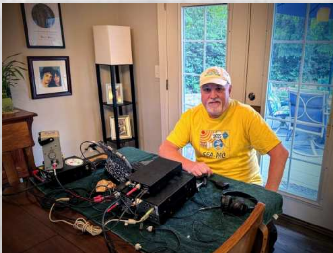
Dave W7UUU at the kitchen table operating desk for the GutterTenna experiment. Radio is an IC-7300 with LDG autotuner. Gutter system is right outside the glass doors.
