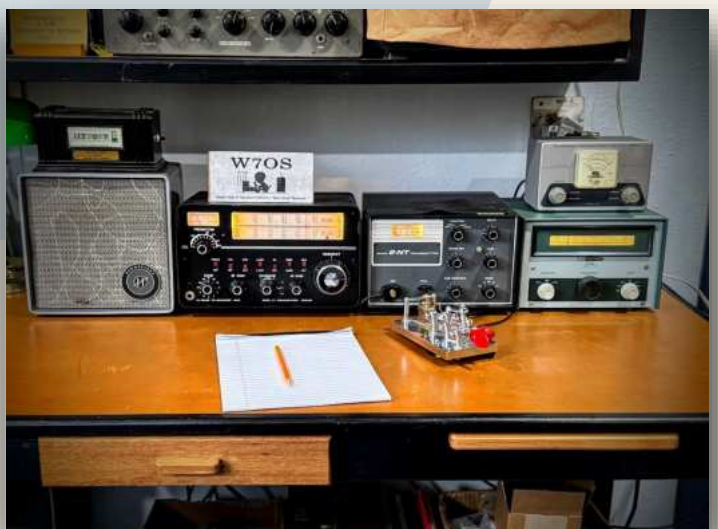
Newly set up in time for the upcoming Classic Exchange and Straight Key Night—drake 2B receiver, 2NT transmitter, and HG-10B VFO
