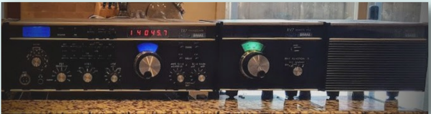
Drake TR-7 transceiver lineup with external VFO and speaker, the day I brought it home in October 2017. Arguably the very first transceiver to cover the 30, 17, and 12m WARC-79 bands even before they existed. This rig was lost in my October 2020 shack fire along with countless other great old radios—I never really got a chance to use it much! Photo by Dave W7UUU
