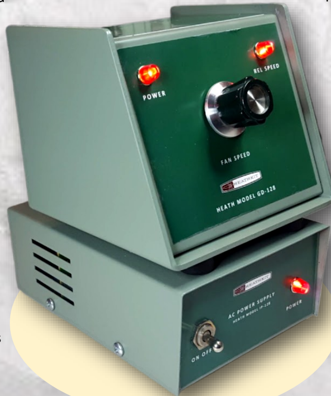
Homebrew "Fake Heathkit" GD-128 Fan Control with equally-fake Heathkit IP-128 power supply.
