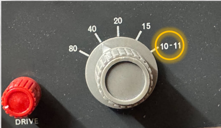
Bandswitch closeup of the Heathkit DX-40 transmitter, showing the combined 10-11 meter band position. All of the Heathkit DX-series transmitters had an 11-meter option, with the DX-100 being the 100-watt pinnacle of the Heathkit 11 meter ham rigs. Photo by Dave W7UUU
