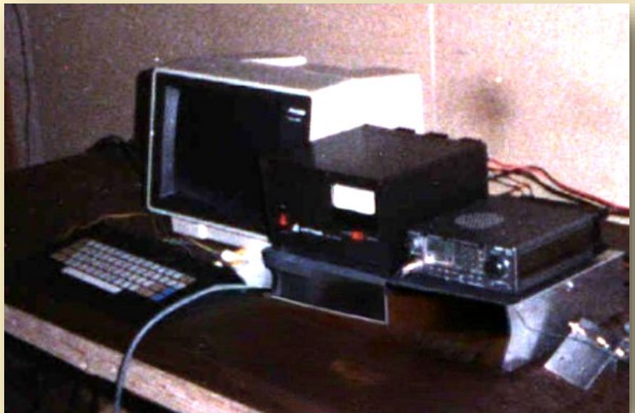
1985 K3LZ-1 packet digipeater owned by KA2DEW and K3LZ . RCA dumb RS-232 terminal with black and white display. Radio is a Kenwood TM-7950 running 45 watts on 2-meters. The TNC (terminal network controller) is here somewhere that makes it all work, but not easy to see in this photo. Photo from TARPN.net
