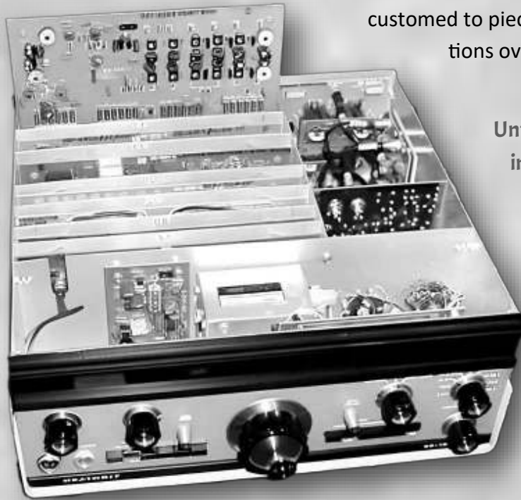
Internal view of the SB-104 showing the plug-in card construction with 13 glass-epoxy PC boards
