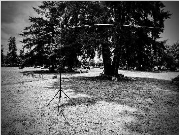
40m NVIS antenna was tried but due to harsh local noise was useless...
