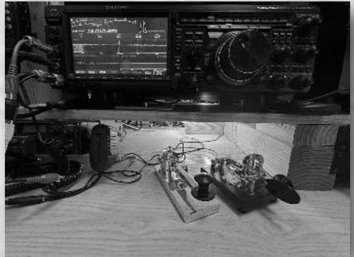
Putikeeg Model 20 Straight Key in my shack—it's connectorized so it can move from my “Big Rig” (FTDX-101MP) to any other rig in the shack
