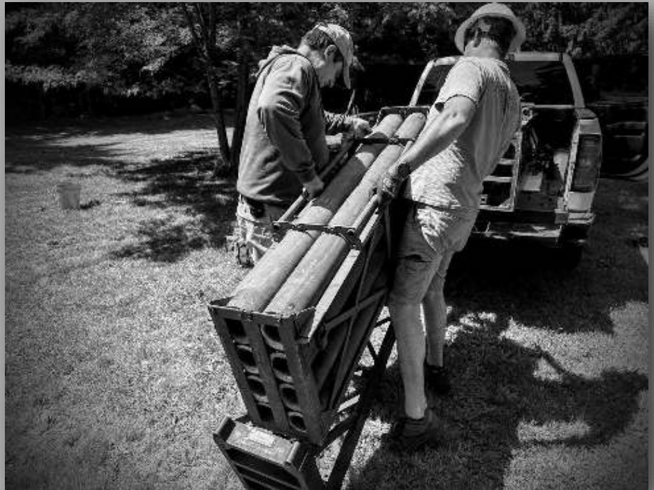
Above: Unloading the AB-577 tower system... called the rocket launcher simply due to the appearance of how the 5-foot tower tubes store in the frame
