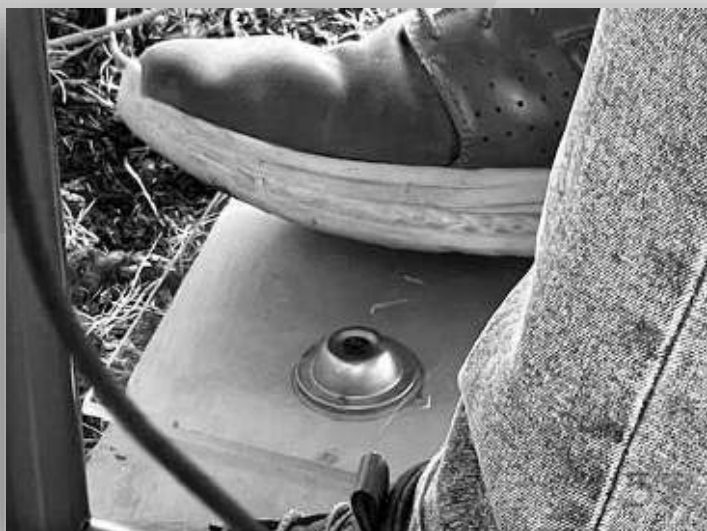
Closeup of Gary WG7X's homebrew footswitch—a doorbell button with a thick Lucite panel to provide a wide activation zone and no slipping!
