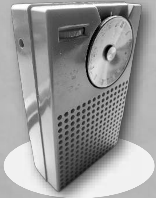
The first commercially manufactured transistor radio, the Regency TR-1 from 1954
