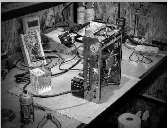
Drake 2B receiver under repair in the W7OS Doc Spike Museum
