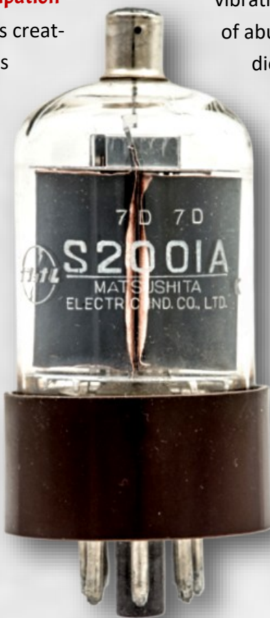
Matsushita S2001A tube, based loosely on the RCA 6146B, widely adopted by Kenwood. Photo by WorldTubeCompany.com
