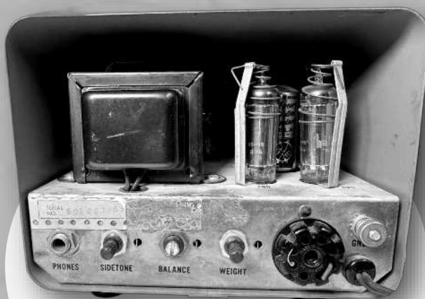
Rear view—you can see the relay between the two regulator tubes. The volume, weight, and balance controls are all "set and forget" on the rear panel.
