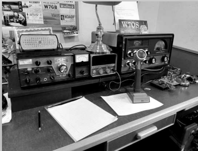
In the primary operating position in the W7OS Museum is the Massive Hallicrafters HT-32A CW/SSB transmitter from 1958, running a full 100 watts on SSB. It's paired with a Drake R4-C receiver for a really great vintage lineup.
