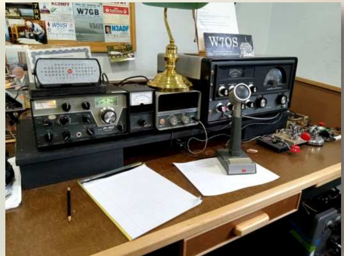
In the primary operating position in the W7OS Museum is the Massive Hallicrafters HT-32A CW/SSB transmitter from 1958, running a full 100 watts on SSB. It's paired with a Drake R4-C receiver for a really great vintage lineup.
