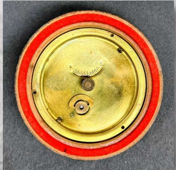
Rearview of the clock, showing time tracking adjustment and winder key
