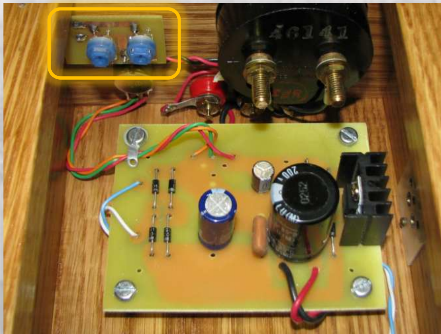
Mounting of the PC boards. Inset: the tiny PCB used to mount the trimmer pots
