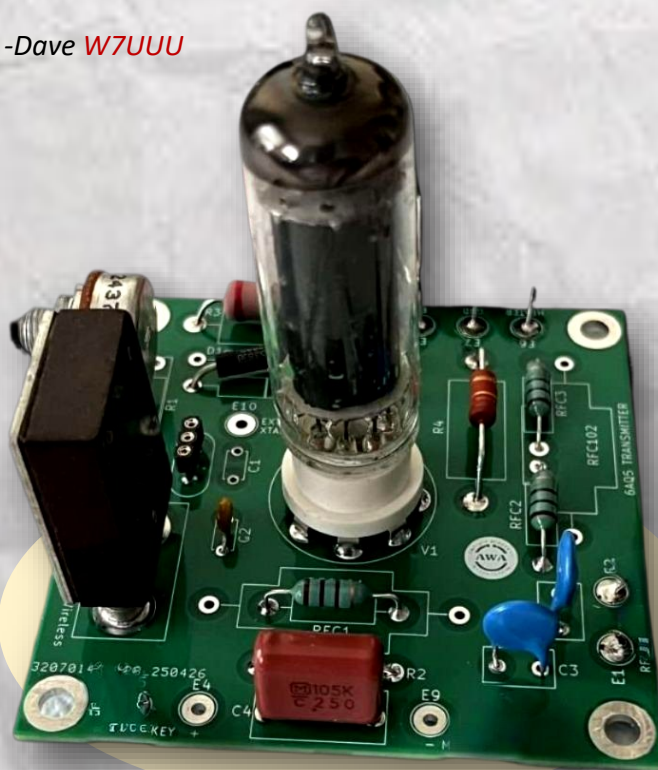
Completed 6AQ5 transmitter as posted on the Antique Wireless Association page Photo by ©AWA 2025
