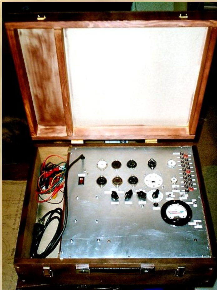
M1KTA homebrew valve tester, photo by M1KTA
