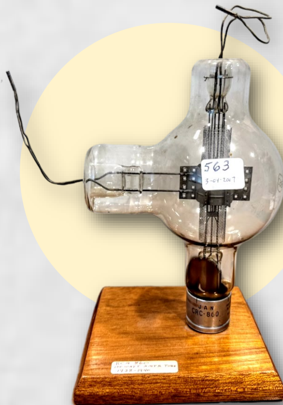
RCA 860 Power Tetrode 100w transmitter tube!
