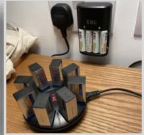
The 130v battery pack shown ready to drop into the slot at the top of the chassis. The rechargeable AA cells provide all filament voltages. Right: the nightly charging ritual!
