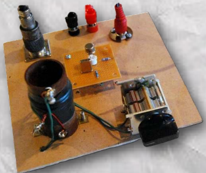
My original Michigan Mighty Mite 1-transistor 20m CW transmitter from a few years ago Photo by Dave W7UUU
