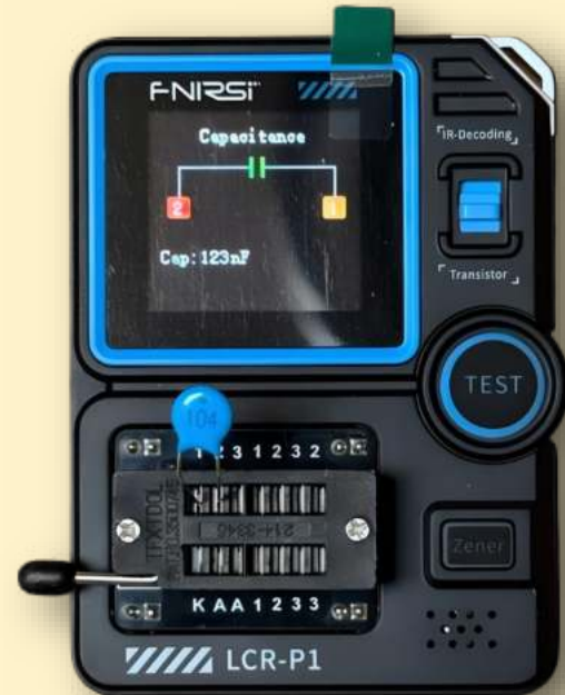
Displaying the test of a mylar disc capacitor
