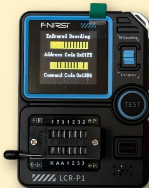
In the IR Decoding mode it will decode IR streams from devices like TV remote controls
