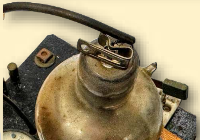
Note the Fahnestock clip used for the anode connection
