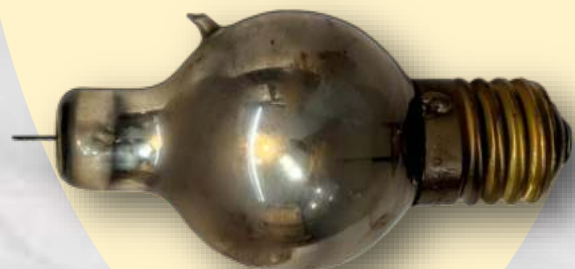
The glass nipple on the side suggests the glass bulb was hand blown. Research confirms this.
