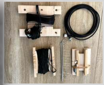
Martin's antenna was an adaptation of an EFHW that he had on hand. He sized it down and used balsa for the winders to reduce weight.
