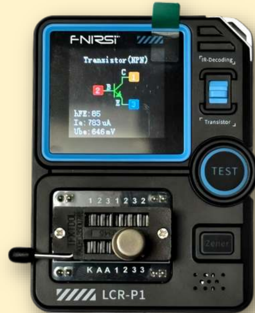
Displaying the test of an NPN transistor. It reads type of transistor, the current gain, the emitter current and the base-emitter voltage
