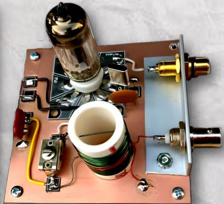
Finished TMMM 1-tube transmitter kit. The yellow wire is soldered to MeSQUARES. Photo from the eBay ad
