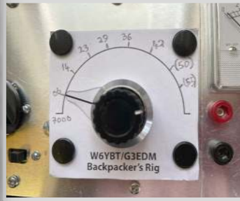
The receiver tuning dial was calibrated to match the exact frequency of the 8 FT-243 crystals that Martin bought on the journey
