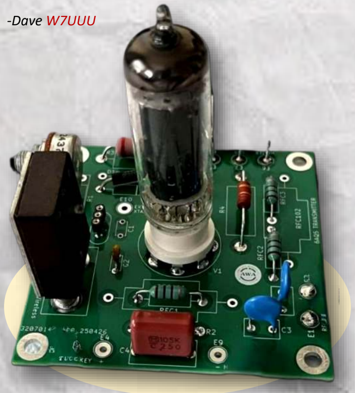
Completed 6AQ5 transmitter as posted on the Antique Wireless Association page Photo by ©AWA 2025
