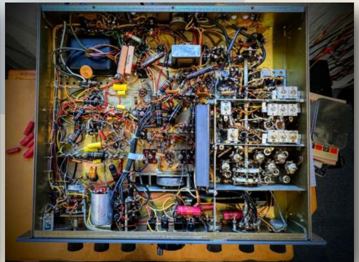
Hallicrafters SX-101A in the midst of a needed recap and realignment by Dan KD7SV
