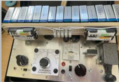
The 130v battery pack shown ready to drop into the slot at the top of the chassis. The rechargeable AA cells provide all filament voltages. Right: the nightly charging ritual!
